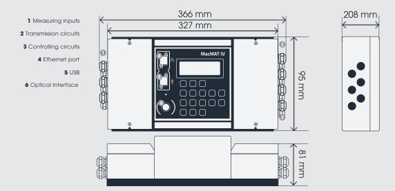
**MacMAT IV** device is equipped with 6 independent, high efficiency communication channels. These channels can work in MASTER or SLAVE mode, that makes possible integration of MacMAT IV with devices and measuring stations systems (chromatographs, dew point converters, controllers) and billings systems SCADA.
